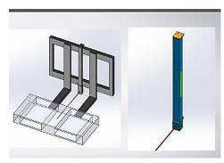
The Laser marker system provides added accuracy and safety. It aligns forks with pallet fork slots to prevent damage to goods/load.
