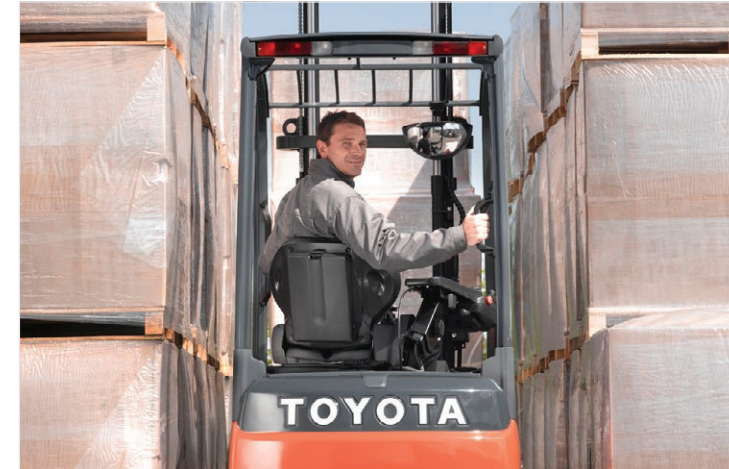
Rear-assist grip enhances reverse travel comfort and productivity by reducing operator back strain. Optional swivel seat facilitates reversing and getting in and out.
