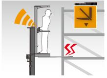
Fork Stuck Descent Stop This detects stuck forks, and warns the operator by visual indicator and sound, thereby ensuring that the platform descends only when the forks are disengaged.
