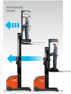
**Automatic Vehicle-speed Control** This controls vehicle speed as well as acceleration and deceleration according to lift height, achieving both stable travel and good productivity.
