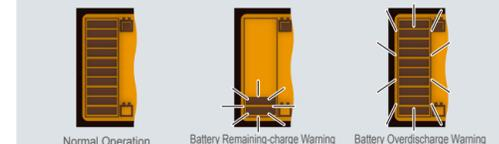
**Battery Remaining-charge Warning and Battery Overdischarge Warning**
