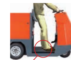
Floor Switch or Seat Switch detects the presence of the operator.
