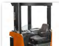
Three different kinds of seats are available, to suit all applications and drivers: Standard basic, Medium and High backrest.
